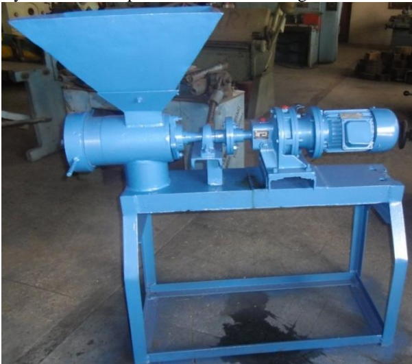
Fig.2. Prototype pelletizer as fabricated
