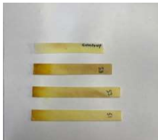
Fig. 9. Indicator paper showing Brown colouration.
