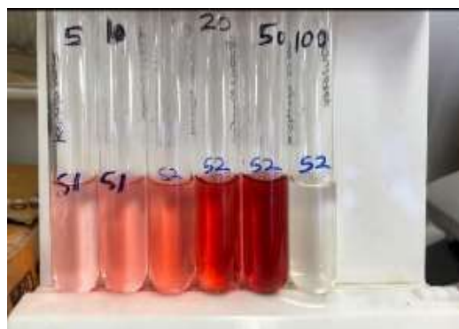
Fig. 1. Standard dilution tubes of IAA (Indole-3-Acetic acid). Fig. 2. S1,S2, S3 tubes showing pink coloration indicating IAA production.
